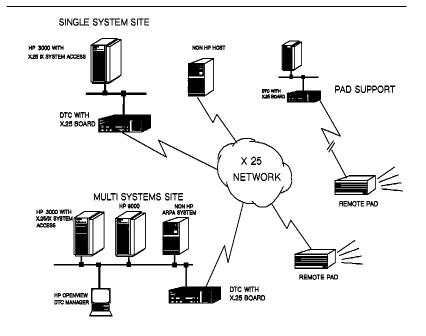
optimized Network Access card in the DTC. The LAN-based architecture of the DTC allows multiple HP 3000/900 hosts to share the same X.25 line, making cost-effective use of the X.25 network subscription.
